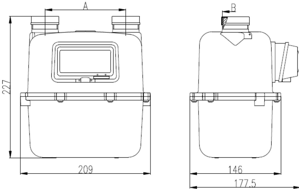
**Dimensions Diaphragm gas meter Atmos® HP G4A**
